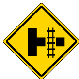
Uncontrolled rail crossing on side road sign
